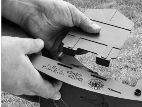
4. Install splash plate.
